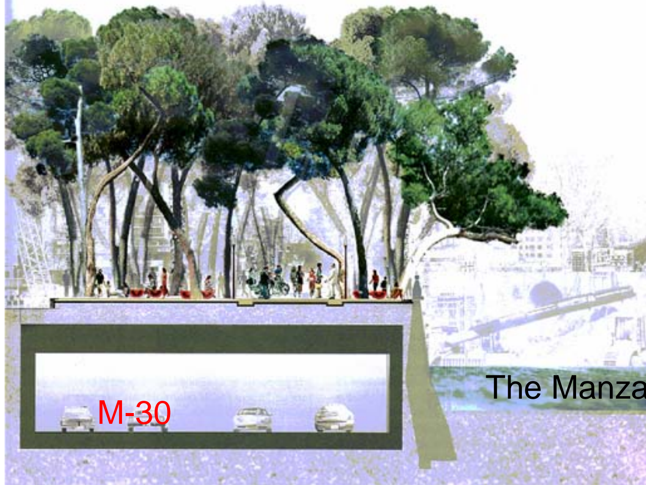
Fig. 3.4. Section of the riverside park from MDRID M-30 (Madrid: Turner, 2007)
